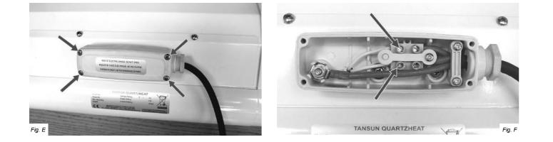
3. Disconnect the emitter from the connector blocks by unscrewing the screws highlighted above in Fig. F and remove the white coloured emitter wires from the terminal block.
