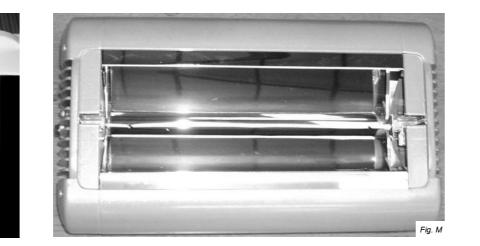
9. The emitter should now be removed from the heater as shown in Fig. M.
