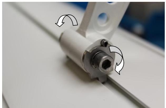
6) Screw 2 cylinder head screws M5x12 (1 spring ring  $\varnothing$  6mm each) through clamping slide with supporting tube attachment on both sides (5mm Allen key)
