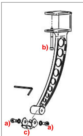
Optional mounting of IR heat radiator SOLAMAGIC 4000 ECO + possible with 2 supporting tube attachment for awning supporting tubes (without additional mounting bracket).
