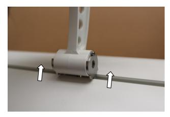
5) Set IR heat lamp with clamping slide at supporting tube attachment. Position of the clamping slide can be adjusted with an Allen key 3mm if necessary.
