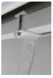
3) Screw closed supporting tube attachment with cylinder-head screw M4x50 (with washer) to the awning supporting tube (4mm Allen key)
