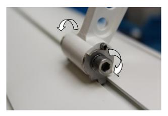
6) Screw 2 cylinder head screws M5x12 (1 spring ring  $\emptyset$  6mm each) through clamping slide with supporting tube attachment on both sides (5mm Allen key)
