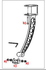
Optional mounting of IR heat radiator SOLAMAGIC 4000 ECO + possible with 2 supporting tube attachment for awning supporting tubes (without additional mounting bracket).
