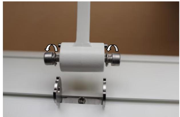
4) Remove allen screws M5x12 (1 spring ring  $\varnothing$  6 mm each) from supporting tube attachments (5mm Allen key)
