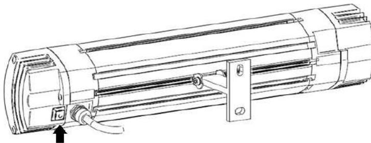
The heating power is activated by operating the switch or the remote control.
