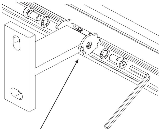
Stop pin opposite cable side, cross hole at the bottom
