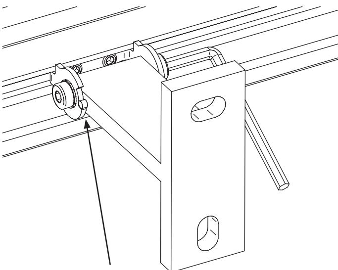
Stop pin on the cable side, cross hole in the front
